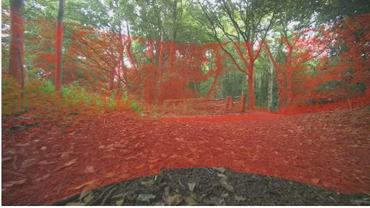
Fig. 6. Evaluation of LiDAR-to-camera calibration: the 3D point cloud captured by the OS-128 LiDAR is projected onto the 2D image plane (shown in red) of the left image from the ZEDx stereo camera.
