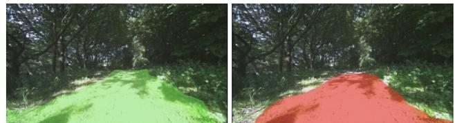
(b) Image with annotated traversable trail ground truth (green). (c) Image with predicted traversable trail (red).
